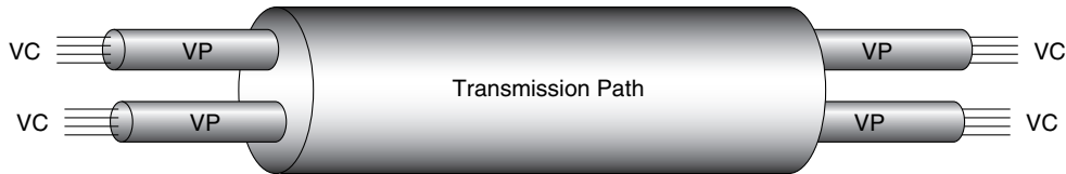
Figure 12-6 VCs Concatenating to Create VPs
