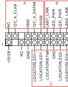
This header supports multiple functions on the front panel, including front panel SMB, internet status indicator.
