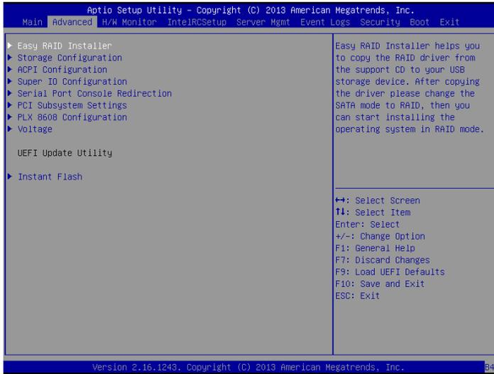
Easy RAID Installer can help you to copy the RAID driver from a support CD to your USB storage device. After copying the RAID driver to your USB storage device, please change “SATA Mode” to “RAID”, then you can start installing the OS in RAID mode.
