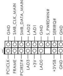
This connector supports Trust-eed Platform Module (TPM) system, which can securely store keys, digital certificates, passwords, and data. A TPM system also helps enhance network security, protects digital identities, and ensures platform integrity.
