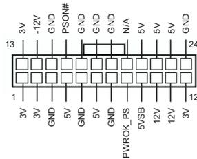
Please connect an ATX power supply to this connector. Though this motherboard provides a 24-pin ATX power connector, it can still work if you adopt a traditional 20-pin ATX power supply. To use a 20-pin ATX power supply, please plug your power supply along Pin 1 and Pin 13.
