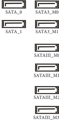
These eight Serial ATA3 (SATA3) connectors support SATA data cables for internal storage devices. The current SATA3 interface allows up to 6.0 Gb/s data transfer rate.
