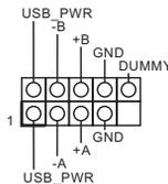
Besides two default USB 2.0 ports on the I/O panel, there is one USB 2.0 header on this motherboard. Each USB 2.0 header can support two USB 2.0 ports.
