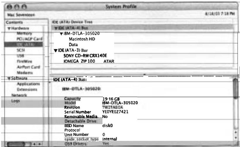
In this example, there are two ATA buses. The first bus has one device connected to it—an IBM hard drive; the second has two devices—a Sony CD-RW drive and an Iomega Zip drive.
