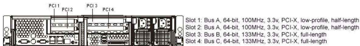
Figure 30. xSeries 346 rear view
