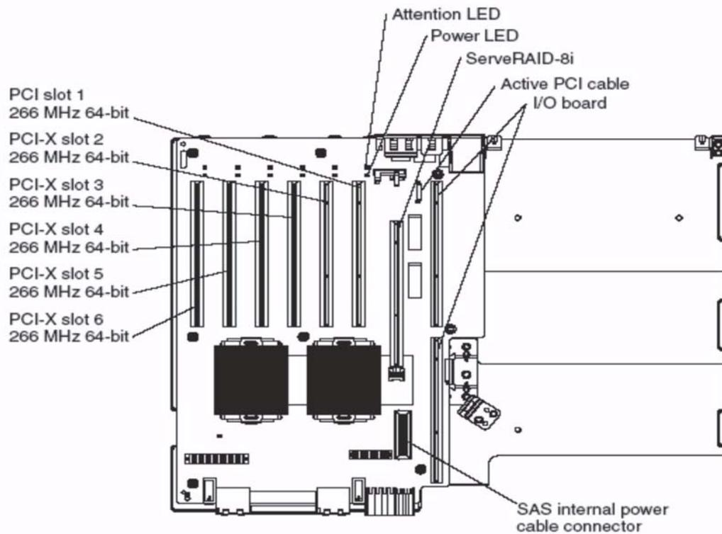
Figure 47. x3950 and x460 system board
