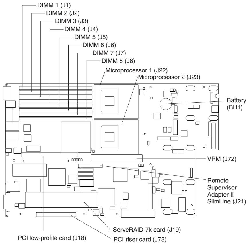
Figure 28. xSeries 346 system board
