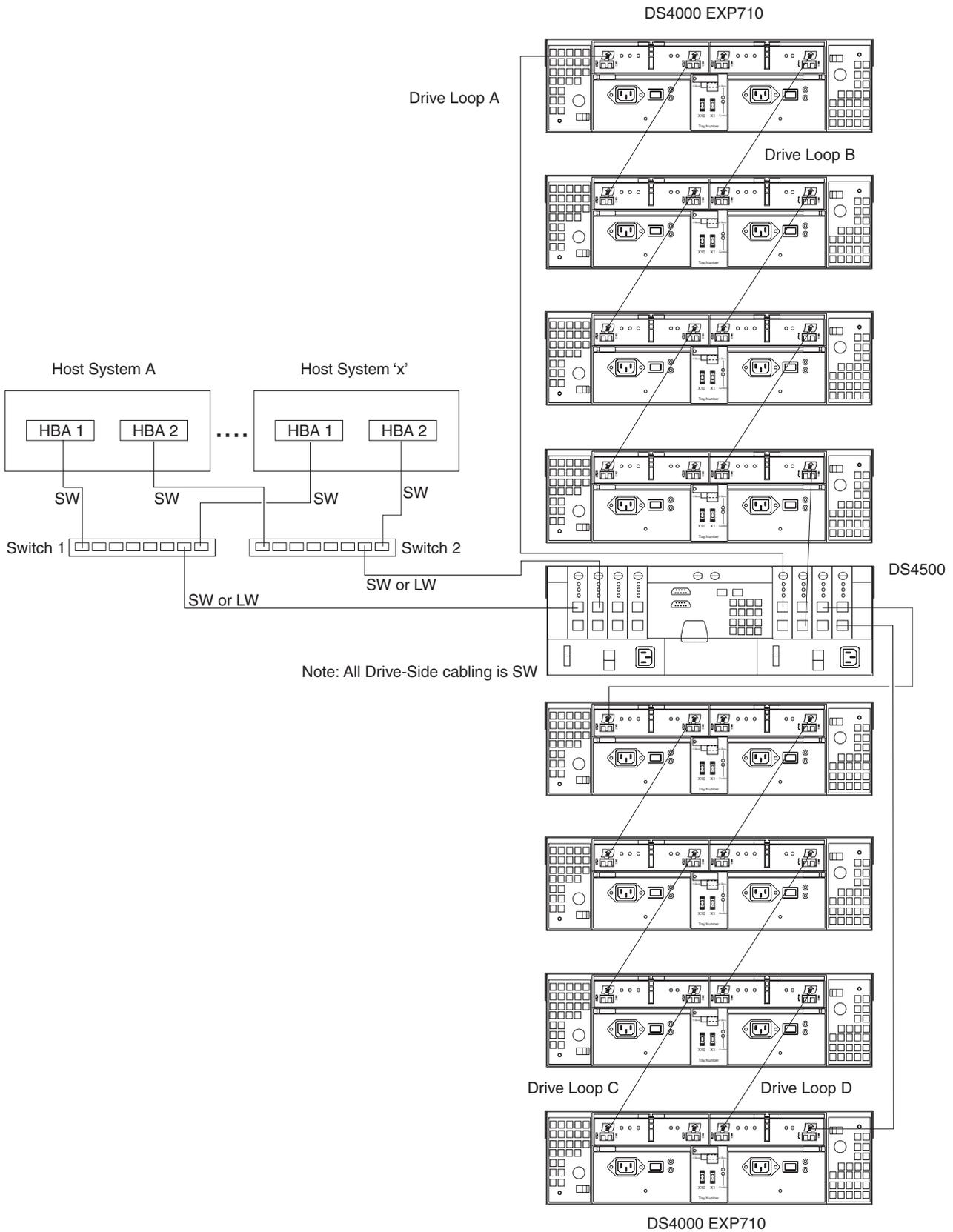
Figure 100. DS4500 Host and Drive Attach Examples
