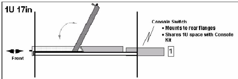
Figure 101. 1U 17in Flat Panel Monitor Console Kit
