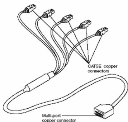
**Figure 60.** IBM BladeCenter Copper Pass-thru Module Cable
