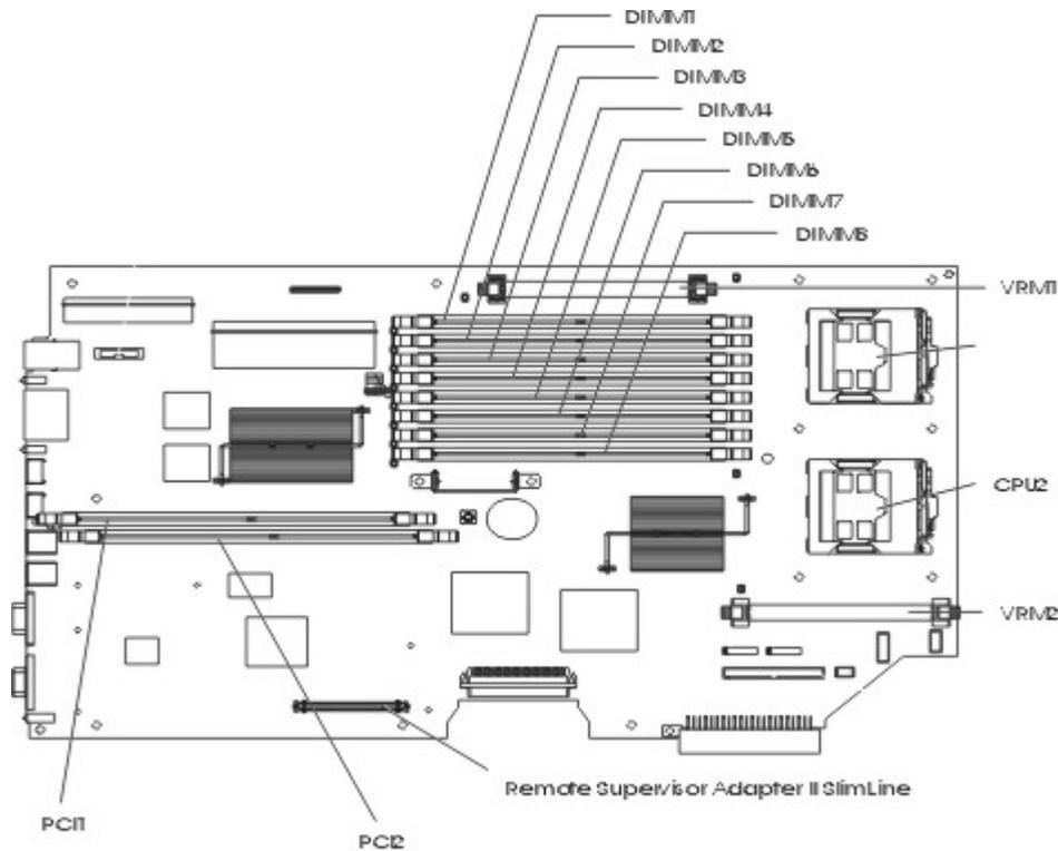
Figure 24. xSeries 336 system board
