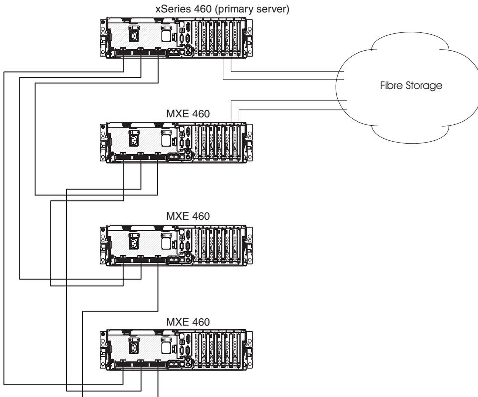
Figure 49. x3950 and x460 Single Node 16-way Configuration
