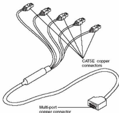
**Figure 67.** IBM BladeCenter Copper Pass-thru Module Cable
