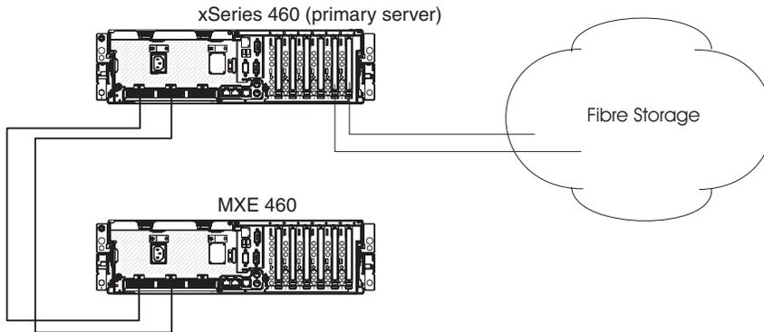
Figure 48. x3950 and x460 Single Node 8-way Configuration
