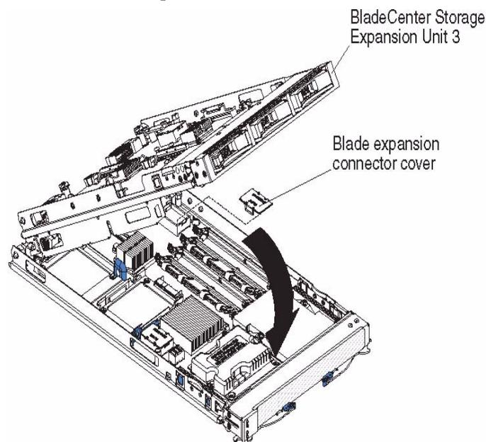
Figure 92. BladeCenter Storage and Expansion Unit 3, View 1
