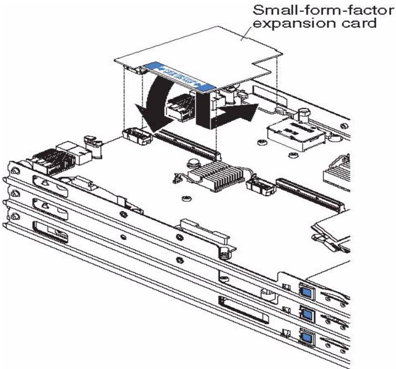
Figure 94. BladeCenter Storage and Expansion Unit 3, View 3
