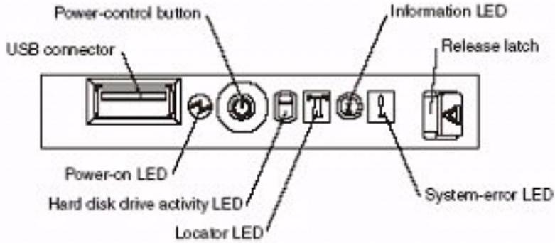
Figure 42. x3850 and x366 operator information panel
