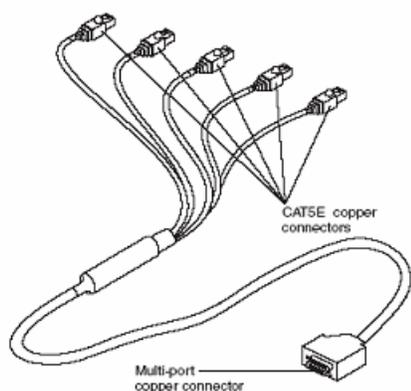
**Figure 53.** IBM BladeCenter Copper Pass-thru Module Cable
