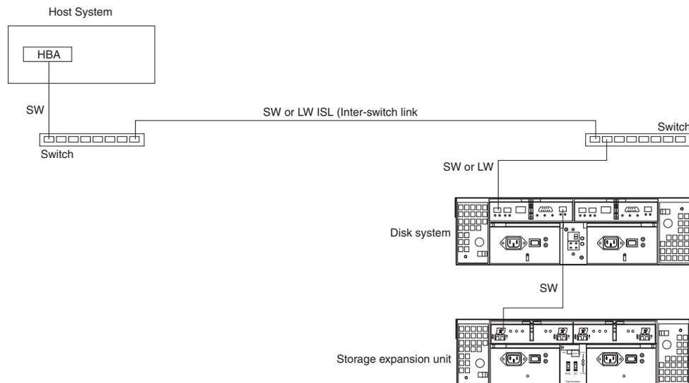
Figure 97. Typical short-wave and long-wave cabling usage
