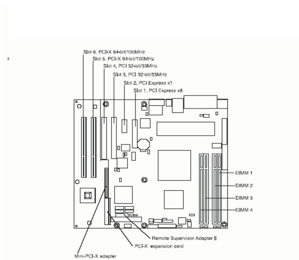
Figure 15. x206m system board
