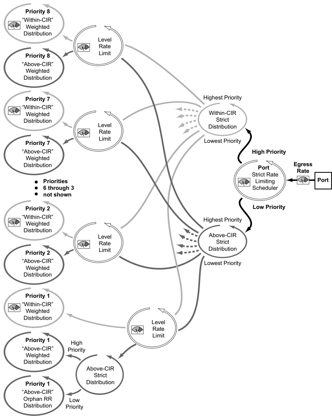
Figure 20 Port Level Virtual Scheduler Bandwidth Allocation Based on Priority and CIR
