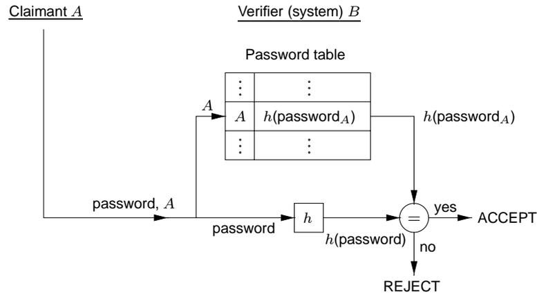
**Figure 10.1:** Use of one-way function for password-checking.
