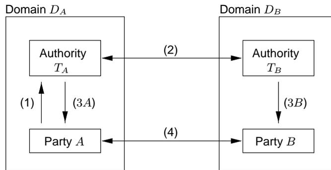
**Figure 13.8:** Establishing trust between users in distinct domains.
