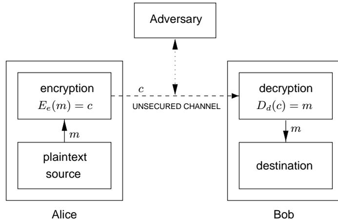
**Figure 1.6:** Schematic of a two-party communication using encryption.
