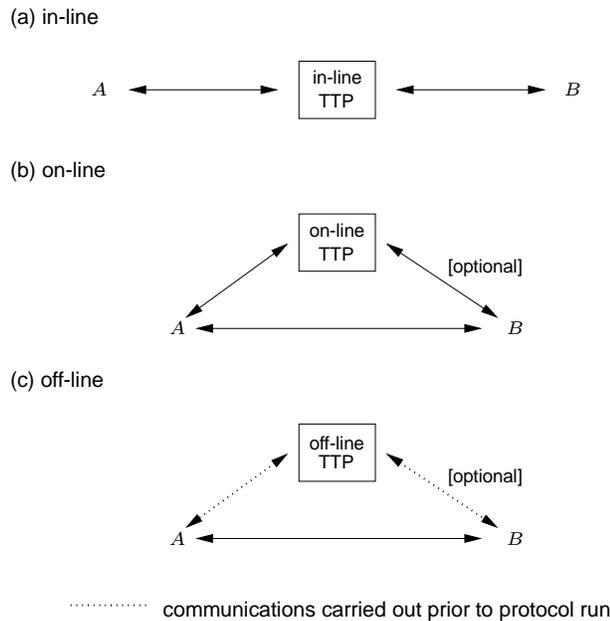
**Figure 13.2:** In-line, on-line, and off-line third parties.
