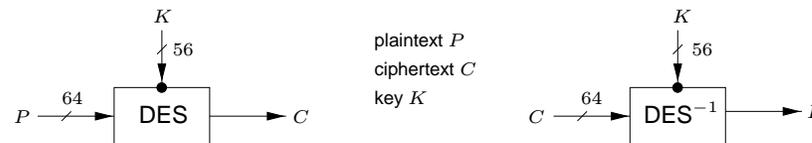
Figure 7.8: DES input-output.
