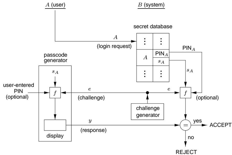
**Figure 10.3:** Functional diagram of a hand-held passcode generator.  $s_A$  is A's user-specific secret.  $f$  is a one-way function. The (optional) PIN could alternatively be locally verified in the passcode generator only, making  $y$  independent of it.
