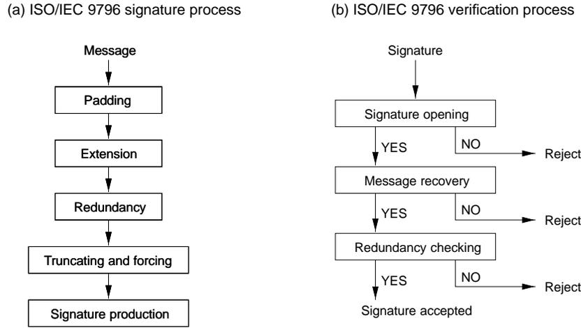
**Figure 11.5:** Signature and verification processes for ISO/IEC 9796.
