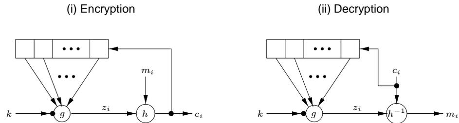
**Figure 6.3:** General model of a self-synchronizing stream cipher.
