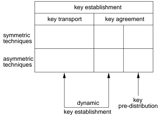
**Figure 12.1:** Simplified classification of key establishment techniques.
