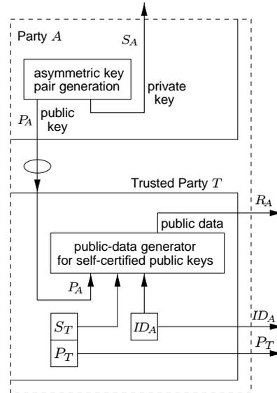
Figure 13.7: (cont'd) Key management in different classes of asymmetric signature systems.
