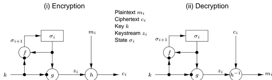
**Figure 6.1:** General model of a synchronous stream cipher.
