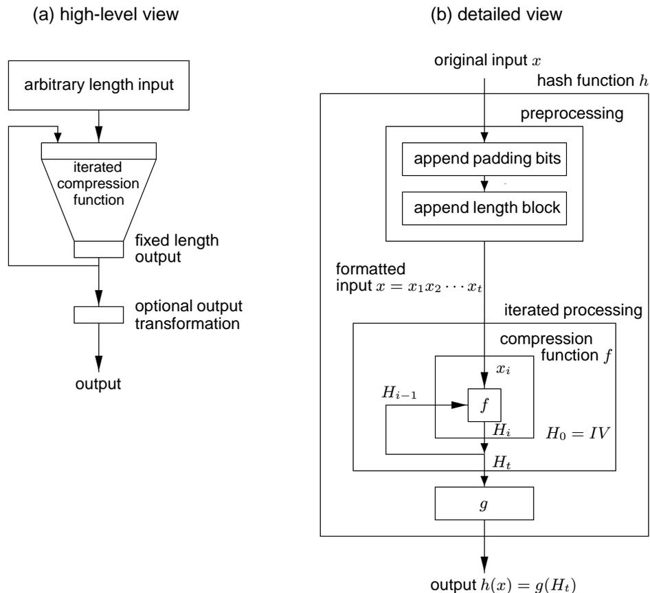
**Figure 9.2:** General model for an iterated hash function.
