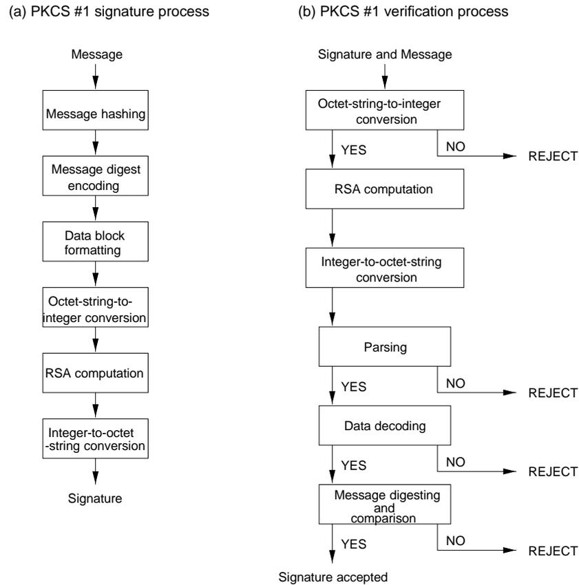
**Figure 11.6:** Signature and verification processes for PKCS #1.
