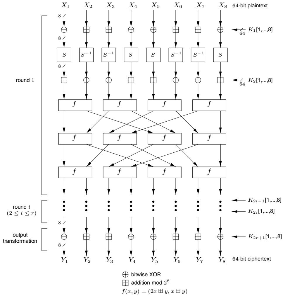
Figure 7.12: SAFER K-64 computation path ( $r$  rounds).
