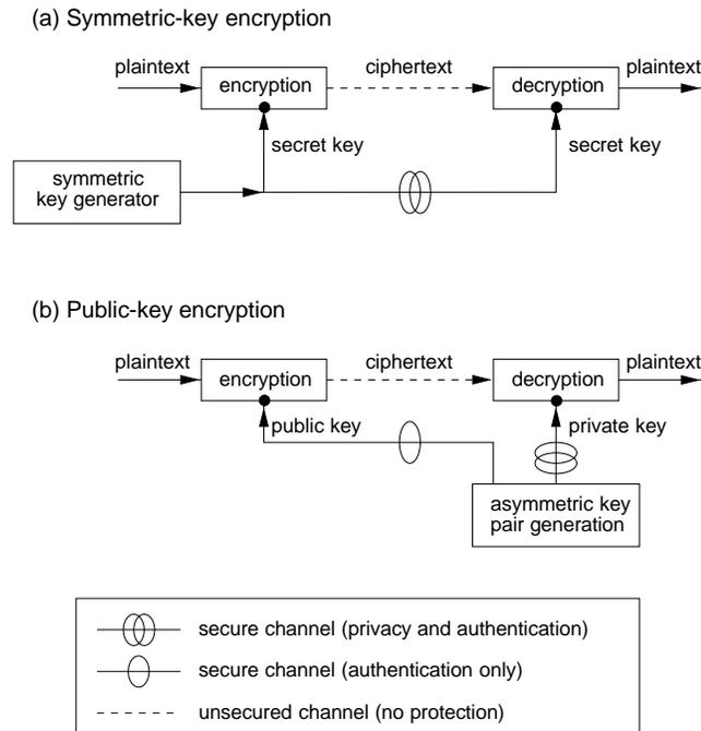
**Figure 13.4:** Key management: symmetric-key vs. public-key encryption.
