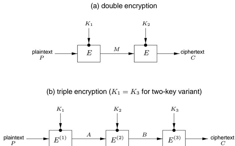
**Figure 7.2:** Multiple encryption.
