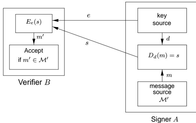
**Figure 1.14:** A digital signature scheme with message recovery.
