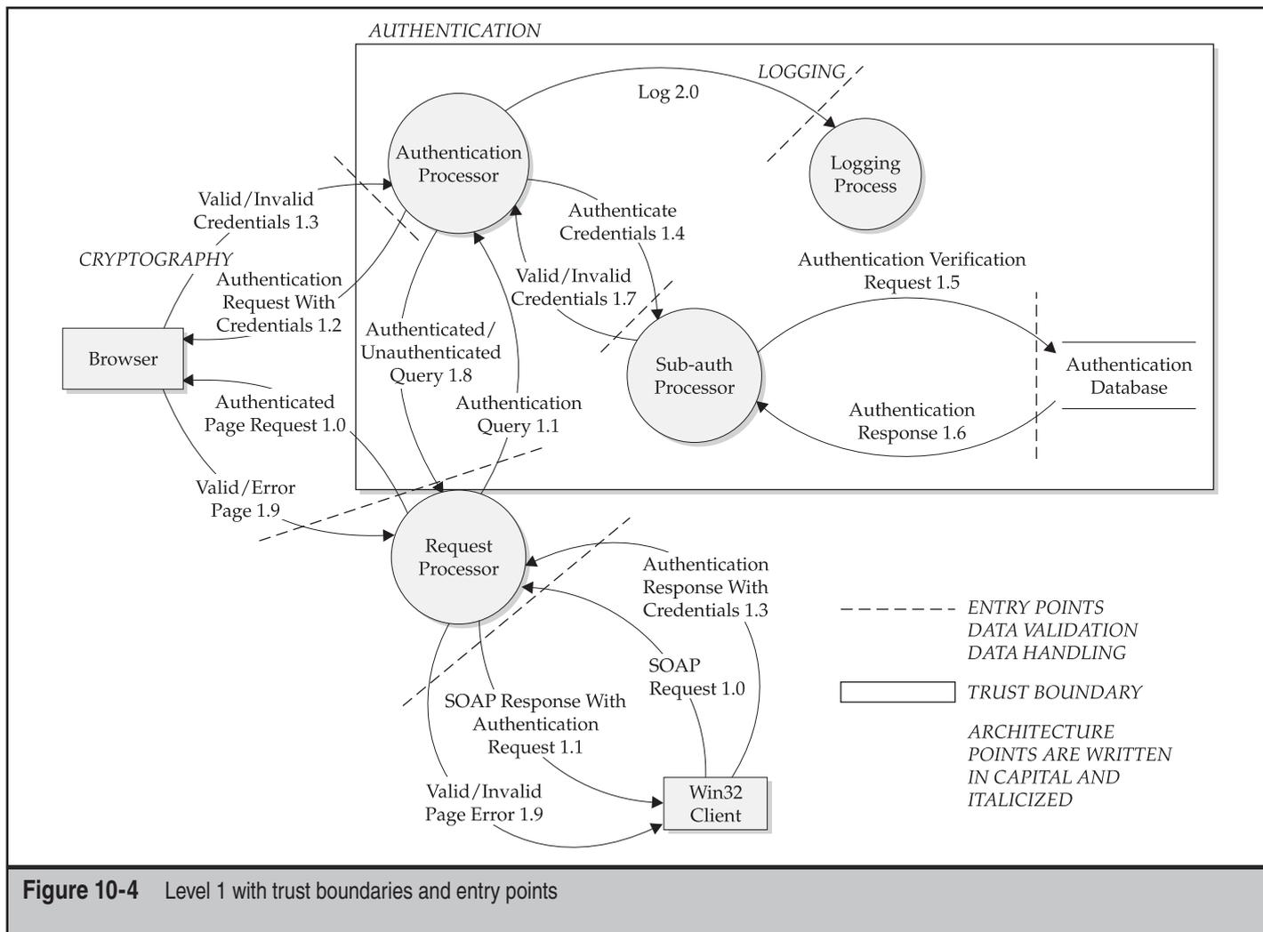
**Figure 10-4** Level 1 with trust boundaries and entry points
