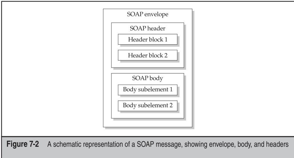
**Figure 7-2** A schematic representation of a SOAP message, showing envelope, body, and headers
