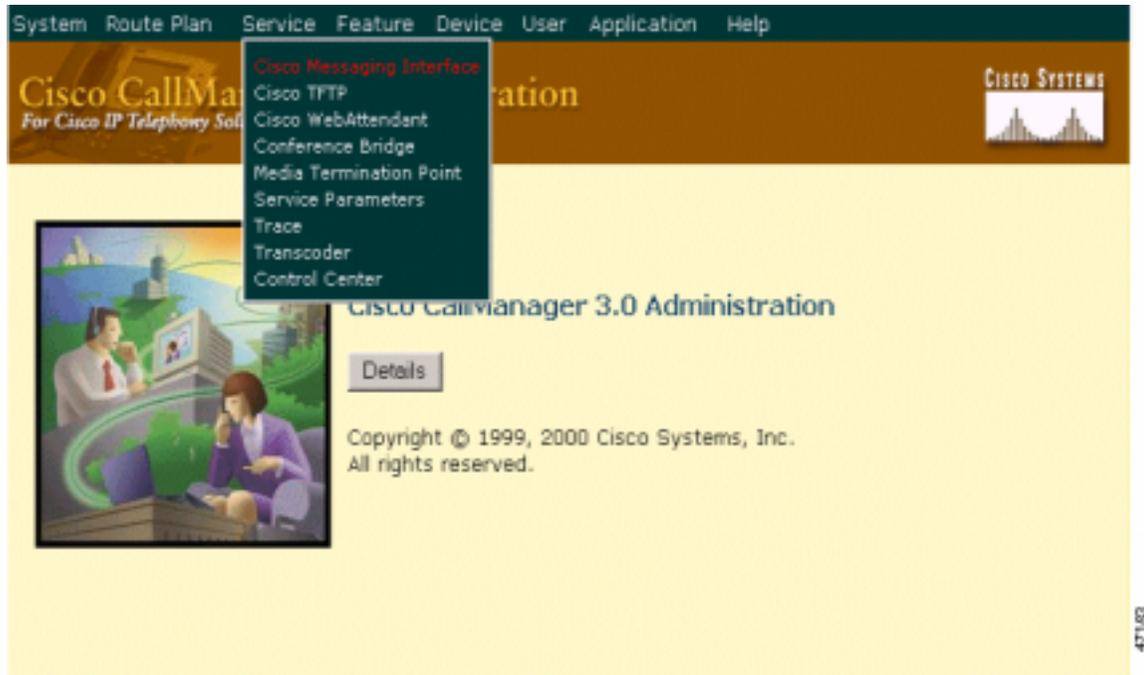
CMI will function in a cluster but can only reside on a single server within a cluster. For example, you cannot have two CMI applications connected to the same voice mail system running at the same time.
