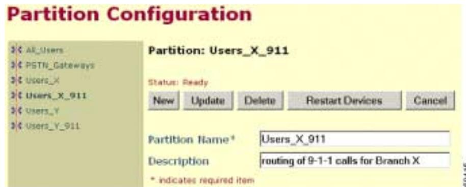
Figure 5-3 shows how the partition should then be included in the calling search space for users located in Branch X.
