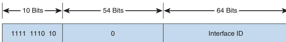
**Figure 2-3** IPv6 Link-Local Address Format
