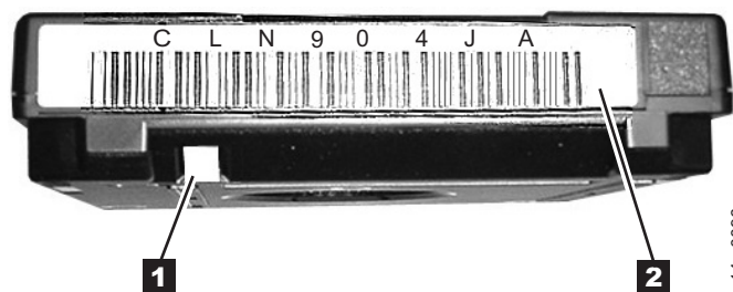
Figure 51. Characteristics that identify the 3592 Cleaning Cartridge
