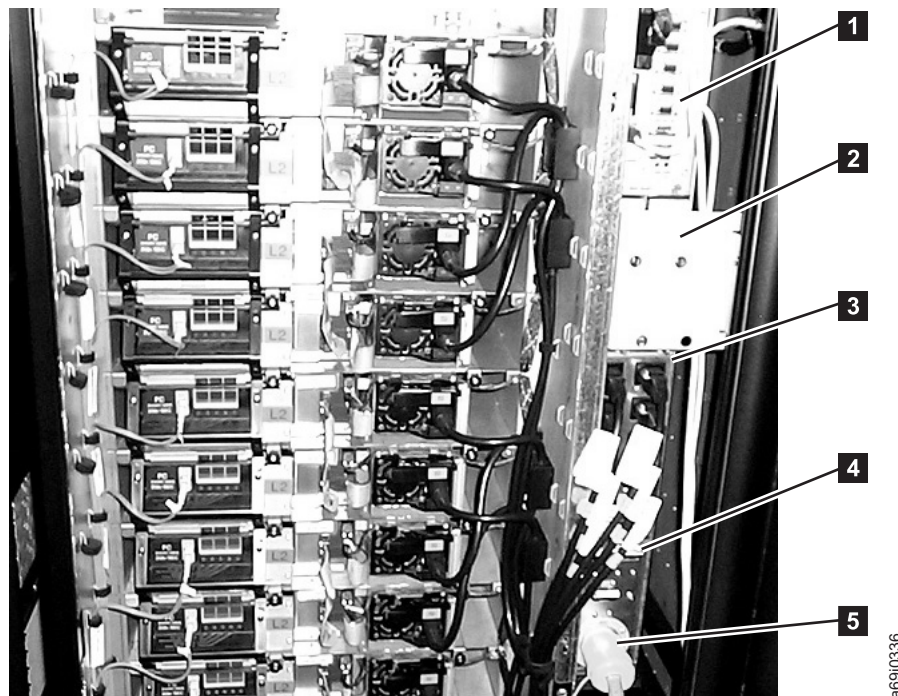
Figure 63. Components of the frame control assembly. Located at the right rear of the 3584 Tape Library, this power structure comes with Models L22, D22, L32, D32, L52, and D52. A Model L52 frame is shown.
