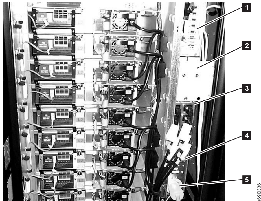
Figure 74. Components of the frame control assembly. Located at the right rear of the TS3500 Tape Library, this power structure comes with models L22, D22, L32, D32, L52, and D52. A model L52 frame is shown.
