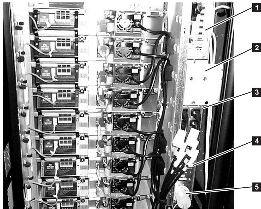
Figure 63. Components of the frame control assembly. Located at the right rear of the 3584 Tape Library, this power structure comes with Models L22, D22, L32, D32, L52, and D52. A Model L52 frame is shown.
