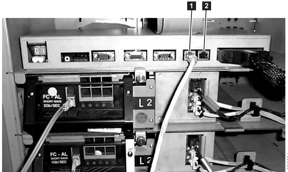
Figure 74. Medium Changer Assembly. The MCA is located above the drives and the power trays, and is part of the enhanced frame control assembly power structure.
