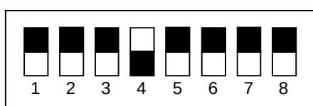
Figure 2.3.1 DIP Switches (Back-up operation to FD is allowed)
