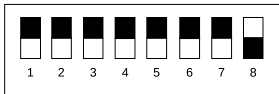
Figure 5.2.3 DIP Switch Setting for Shutting Down CTL ASSY
