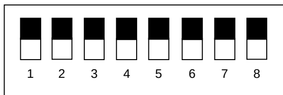
Figure 2.2 Standard DIP Switch Settings
