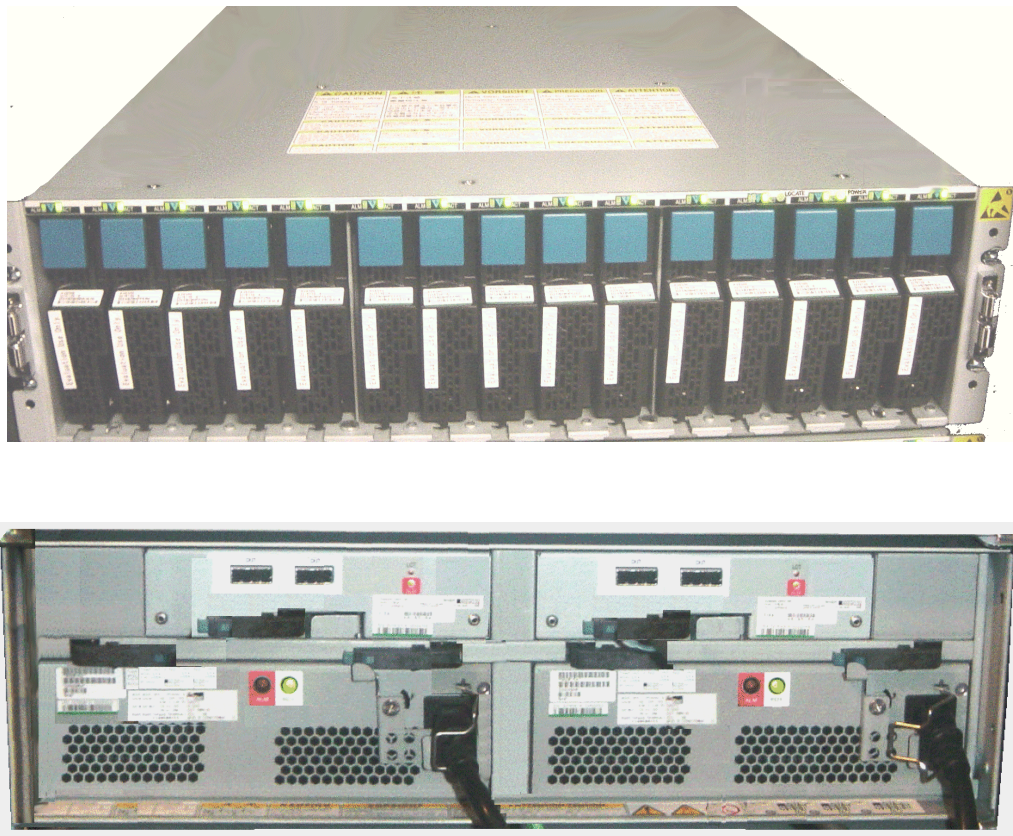
Figure 1-11: AMS 2000 Family Expansion Unit Front and Rear Views
