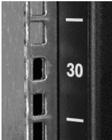
Figure A.1 EIA (U)nit Measurement on Rack
