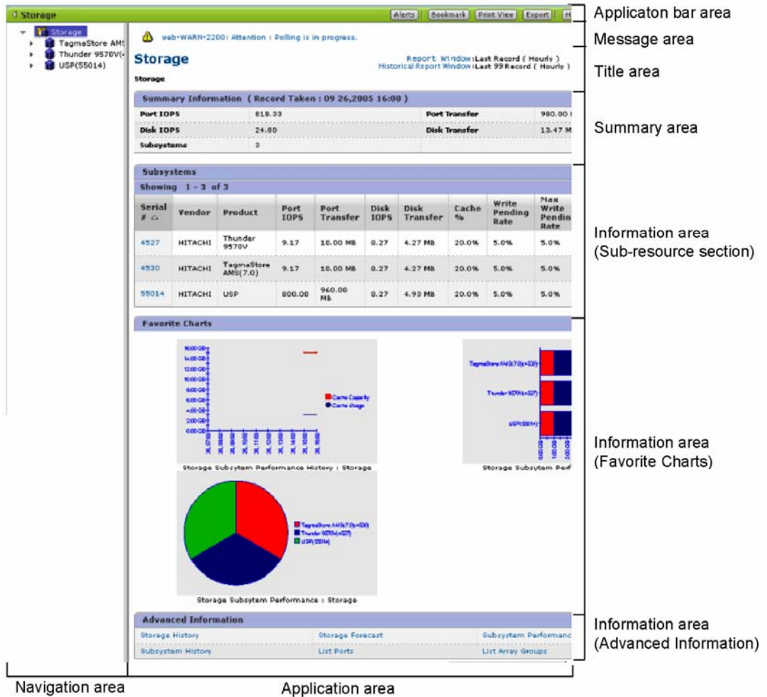
Figure 1.2 The Structure of the Report Area
