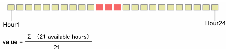
Figure 3.1 Example Aggregation Formula for One Day Interval (Free Space)
