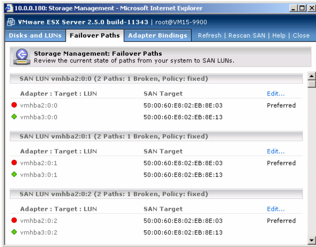
Figure 5.2 Failover Paths of VMware Management Interface
