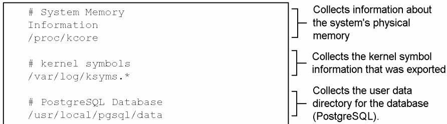
Figure 7.1 Coding Example of a File that Defines the Information to Be Collected
