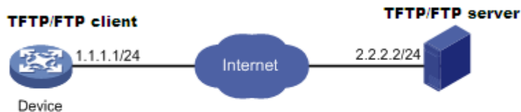
Figure 1 Set up the upgrade environment
