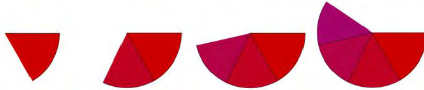
Figure 3.20. Slices of pie being added to the canvas as the for loop iterates through the data array
