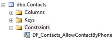
Figure 7-11. A well-named default constraint
