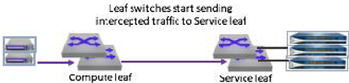
Figure 9-14: Leaf switches intercept
